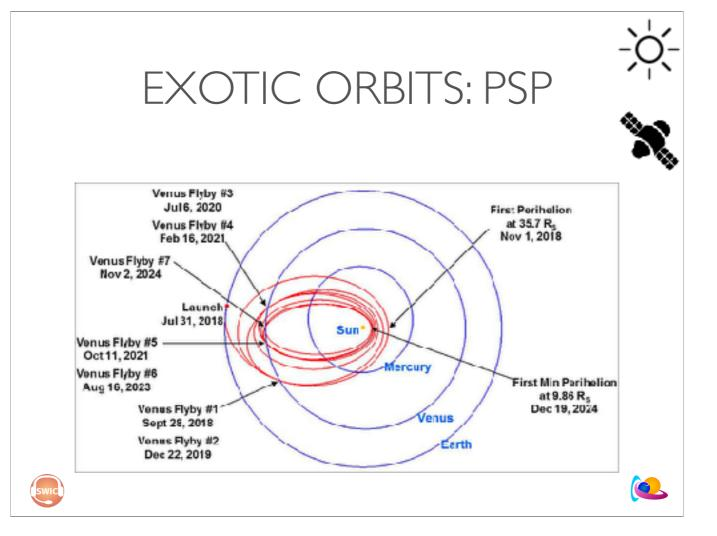
Parker Solar Probe was launched in 2018. The spacecraft will fly through the Sun's atmosphere as close as 6 million km to our star's surface, well within the orbit of Mercury and more than seven times closer than any spacecraft has come before. (Earth's average distance to the Sun is 149 million km.)
