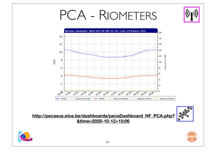
A riometer is an instrument used to quantify the amount of electromagnetic-wave ionospheric absorption in the atmosphere. "opacity" of the ionosphere to radio noise emanating from cosmic origin.
