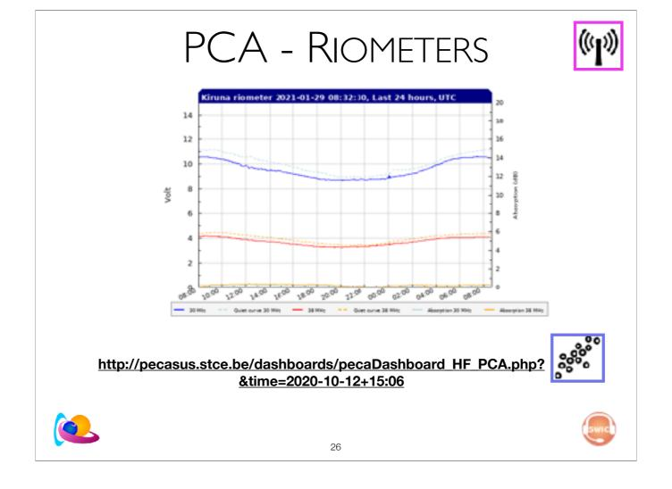
A **riometer** is an instrument used to quantify the amount of electromagnetic-wave ionospheric absorption in the atmosphere. "opacity" of the ionosphere to radio noise emanating from cosmic origin.
