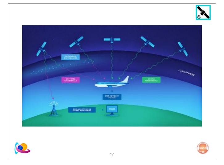
The ionosphere plays also a crucial role in satellite navigation. The signal sent by the satellite has to pass through the ionosphere to reach the receiver. **Solar storms can introduce small scale structures** in the ionosphere. When the signal encounters these obstacles, its amplitude and phase can alter very rapidly. Similarly, when the number of electrons in the ionosphere increases dramatically due to a solar storm, positioning errors are introduced in satellite navigation.
