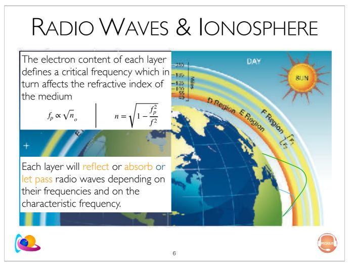
Both GNSS and HF com use radio waves -> how do radio waves behave in an ionised medium
