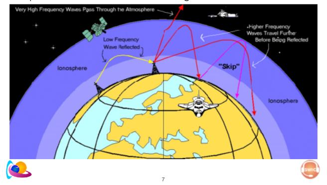
The ionosphere has the ability to reflect radio waves. If the degree of ionisation would be zero, no radio waves would be reflected and all would pass.
