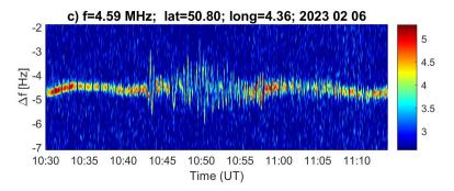
However: only a single frequency is sounded, so no complete electron density profile can be obtained.
