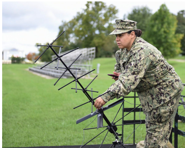
Setting up a satellite communications antenna for a demonstration of the Mobile User Objective System (MUOS)
