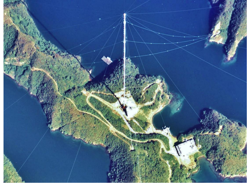
Shushi-Wan Omega Transmitter (station H) of the Omega navigation system (389 m high!)
