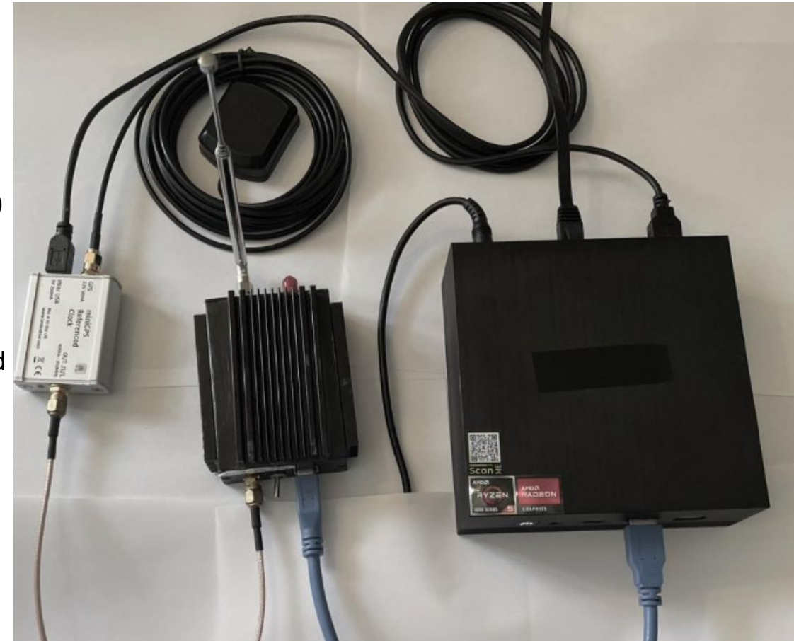
HamSCI Personal Space Weather Station SDR High Frequency Receiver, [36]
