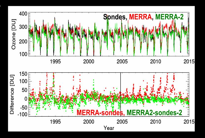
Total ozone derived from South Pole ozonesonde measurements, MERRA, and MERRA-2. The SBUV and MLS/OMI periods are separated. The large excursions arise from limited SBUV coverage.
