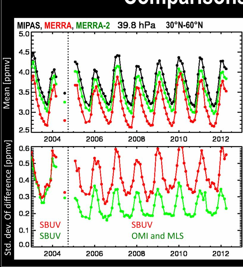
The Michelson Interferometer for Passive Atmospheric Sounding was flown on Envisat, 2002-2012. The top plot shows the 30°N-60°N zonal mean ozone from MIPAS, MERRA and MERRA-2 interpolated to the 39.8 hPa pressure level. Both reanalysis are biased low with respect to MIPAS but the bias is smaller in MERRA-2 at that level.
