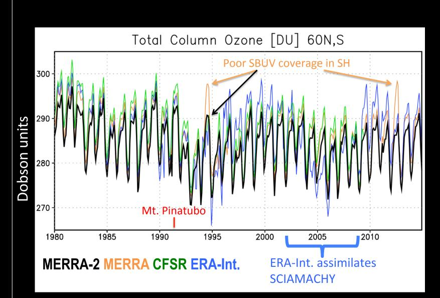
Time series of the 60°S-60°N total ozone from MERRA, MERRA-2, ERA-Interim and CFSR. All assimilate SBUV ozone. In addition, ERA-Int. concurrently uses multiple other data sources and MERRA-2 assimilates MLS/OMI in place of SBUV in the latter period. These features are discernible in all 4 reanalyses:
