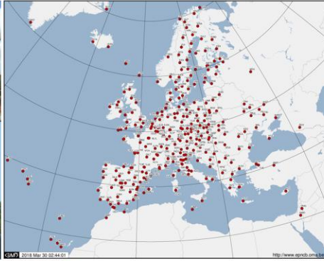
EUREF Permanent GNSS Network
